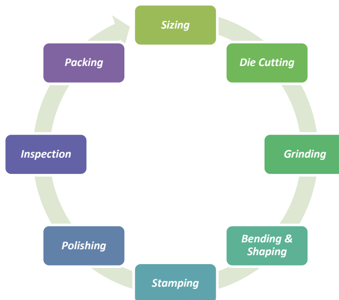
Figure 3: Process Flow Chart of Spoons
