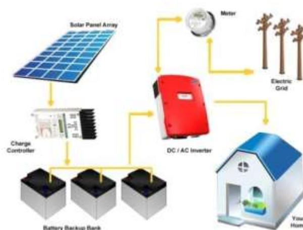
**Fig 02: On-Grid / Hybrid PV System**
