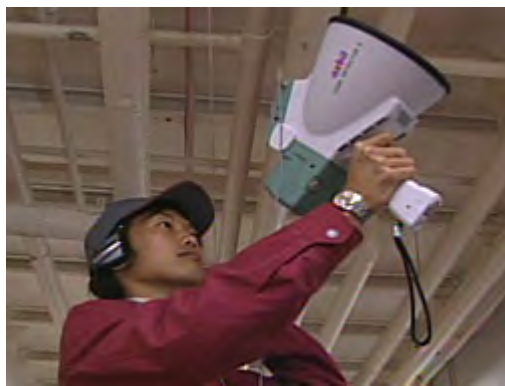
Figure 2-6 Air leak detect by supersonic detector
