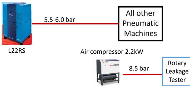
**Figure 2 Installation of high pressure air compressor**
