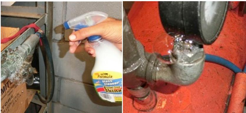
**Figure 1 Soap water inspection and soap bubbles from air leakage pipe joints**
