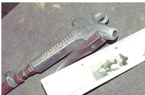
**Figure 1 Air blow gun with 8mm dia. nozzle**
