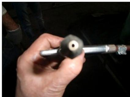
**Figure 2 Air blow gun with 2mm dia. nozzle**
