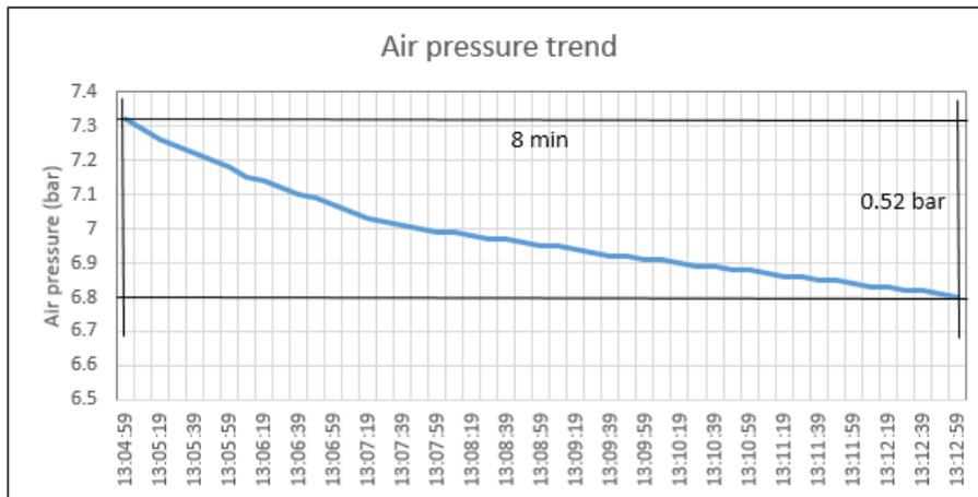
Figure1 Measurement of air pressure reducing trend at outlet of compressor during no air use in plant.
