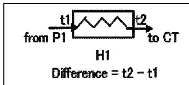
Difference temperature of heat exchanger (H1) before and after to introduce inverter is as follow.
