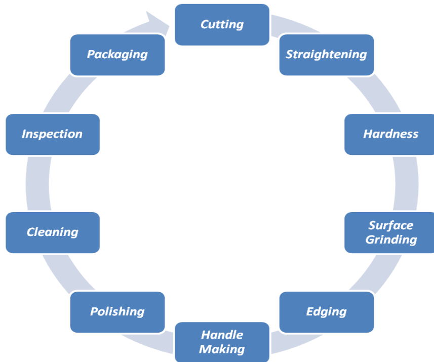
Figure 2: Process Flow Chart for Knives
