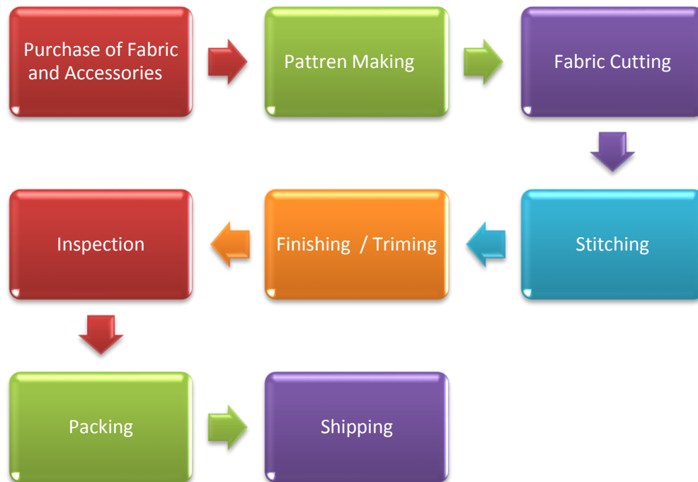
Figure 2: Track Suit Production Process Flow
