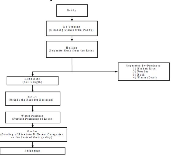
**Figure 1: Production Process Flow**
