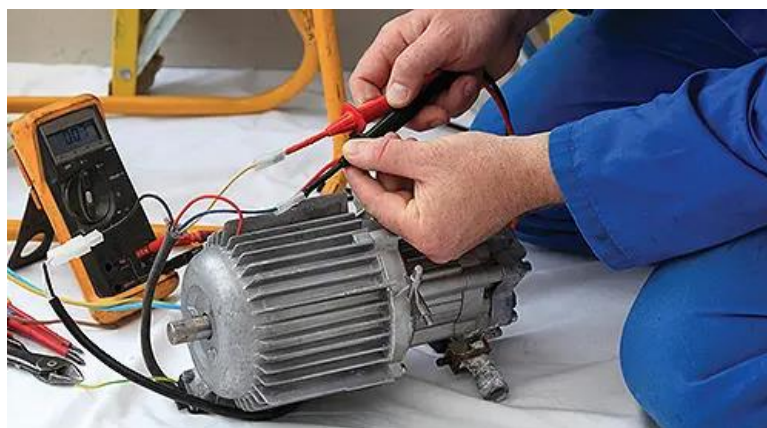
Figure 40: Testing of an Electric Motor
