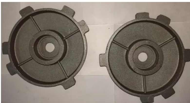
Figure 34: End-Shields of a Motor after Shot Blasting
