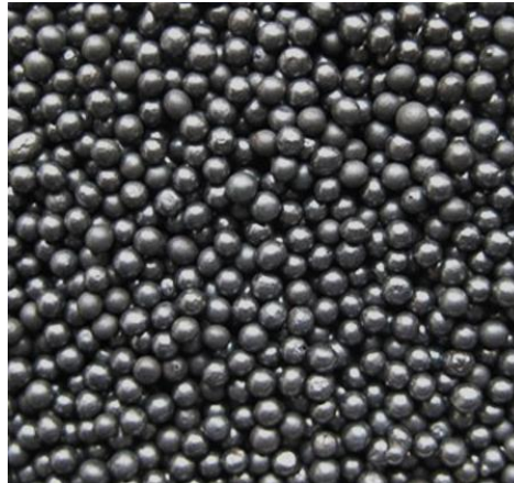
Figure 16: Steel Shots used for Shot Blasting
