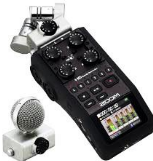
Figure 3: Zoom Device with 4 Microphones
