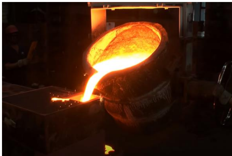
Figure 19: Transfer of Molten Metal
