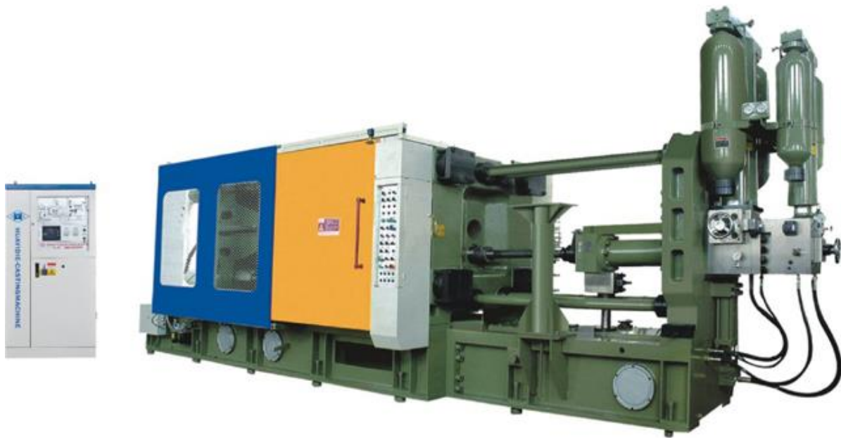
Figure 9: High Pressure Die-Casting Machine
