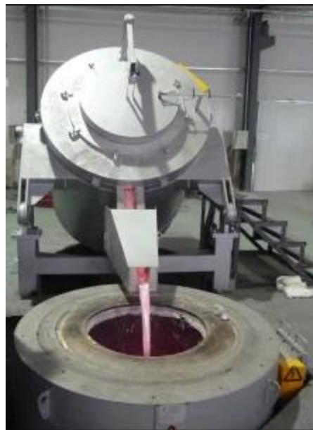
Figure 8: Melting and Holding Furnace
