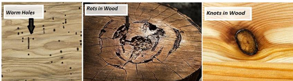
Figure 16: Worm Holes, Rots and Knots in Wood
