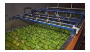
The hot water treatment system comprises of a feeding conveyor, hot water dipping tank, drying system and packing tray. Each component except packing tray is mounted on wheels for ease of transportation. The water tank is made of stainless steel in order to avoid rusting. The water is heated through three gas burners.
