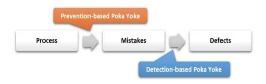
**Prevention Based Poka Yoke:** In this type, system is designed in such a way that that mistakes are impossible to occur. It is a proactive approach in which system acts before a defect occurs.
