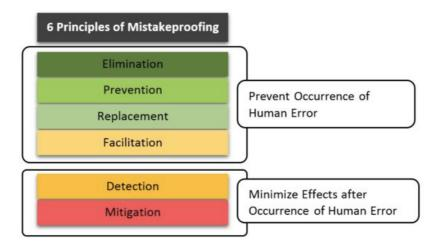
**Elimination, Prevention, Replacement and Facilitation** are to avoid the occurrence of mistakes i.e. **Prevention Based Poke Yoke. Detection and Mitigation** are to minimize the effects of mistakes once they occur i.e. **Detection Based Poka Yoke.**
