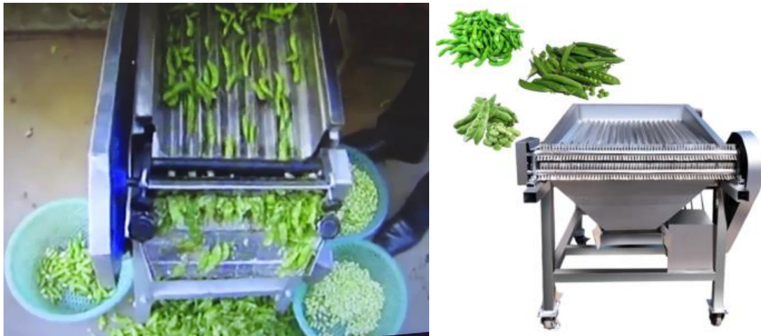
Figure 16: Peas Shelling Process
