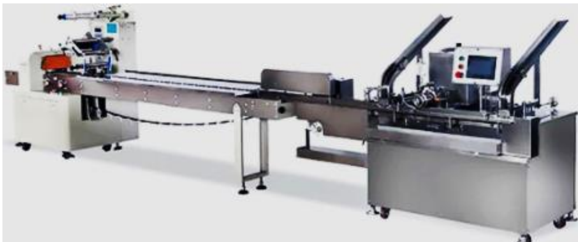
Figure 7: Automatic Production line - Cookies
