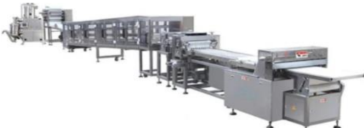
Figure 3: Automatic Production Line - Chocolate
