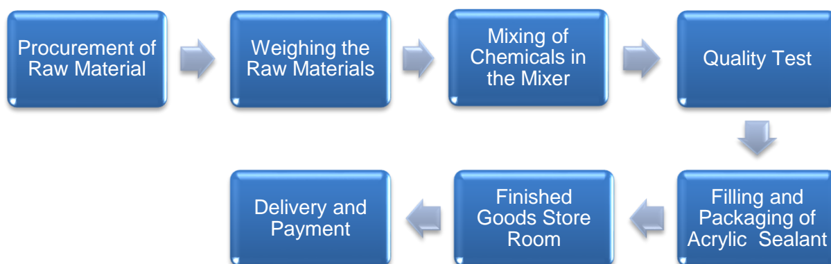
Figure 19 : Process Flow for Manufacturing of Acrylic Sealant
