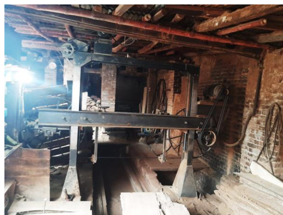
Figure 3 Peeling of Logs by Horizontal Band Saw Machine
