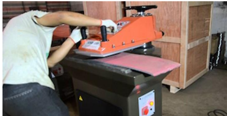
Figure 7: Hydraulic Press (Clicker) Machine
