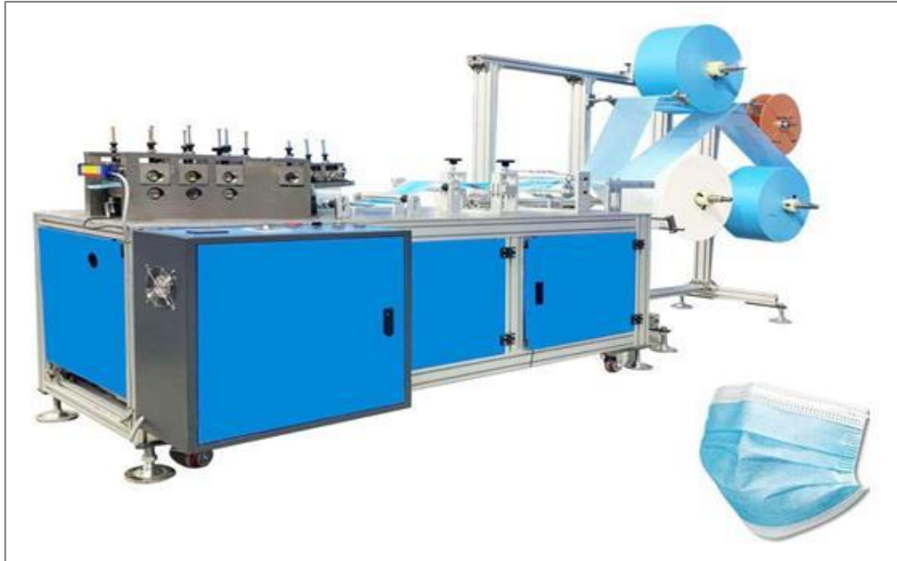
Figure 2: Disposable Surgical Mask Manufacturing Machine
