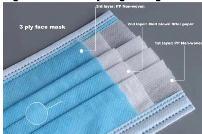
Figure 12: Textile Layering of Surgical Mask
