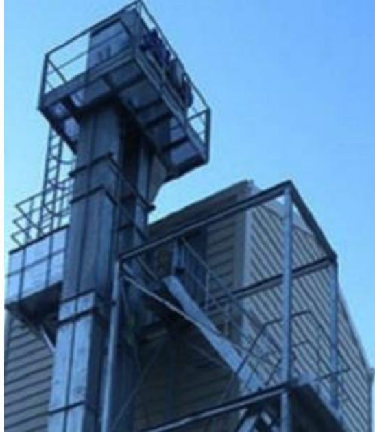
Figure 6: Lifting of Crushed Material Using Bucket Elevator
