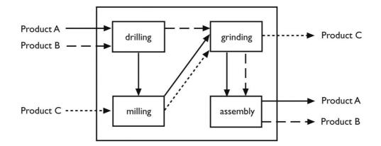
Figure 3: Example-Process Focused Layout
