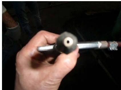
Figure 2 Air blow gun with 2mm dia. nozzle
