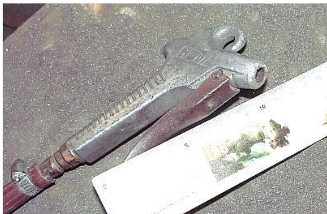
Figure 1 Air blow gun with 8mm dia. nozzle
