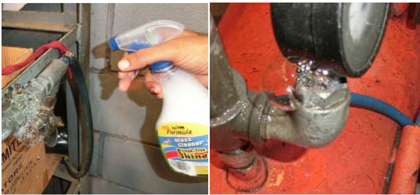
Figure 1 Soap water inspection and soap bubbles from air leakage pipe joints
