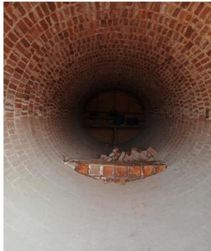
Temperature inside the furnace is maintained in the range 830-950C. The chemical reaction taking place in the furnace is as follows:
