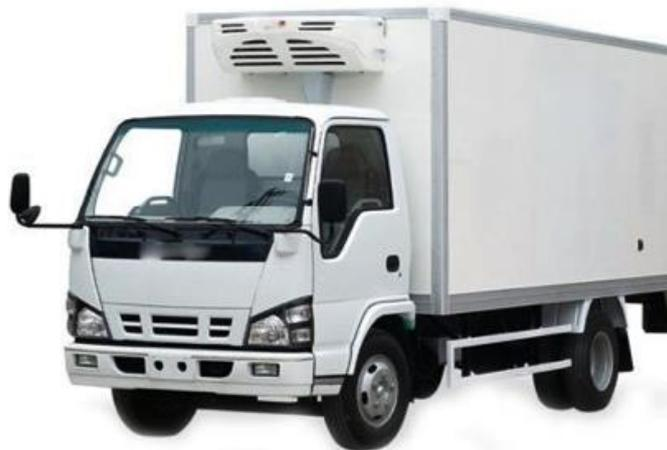
The study has been carried out assuming one reefer truck with a diesel engine of 2,771cc displacement and payload capacity of 3,350 kilograms; equipped with an insulated container of external dimensions 168'x74'x82' (length x width x height); with a loading capacity of 3 tons. Further assumptions regarding products to be transported and the related requirements are given in Table 1.
